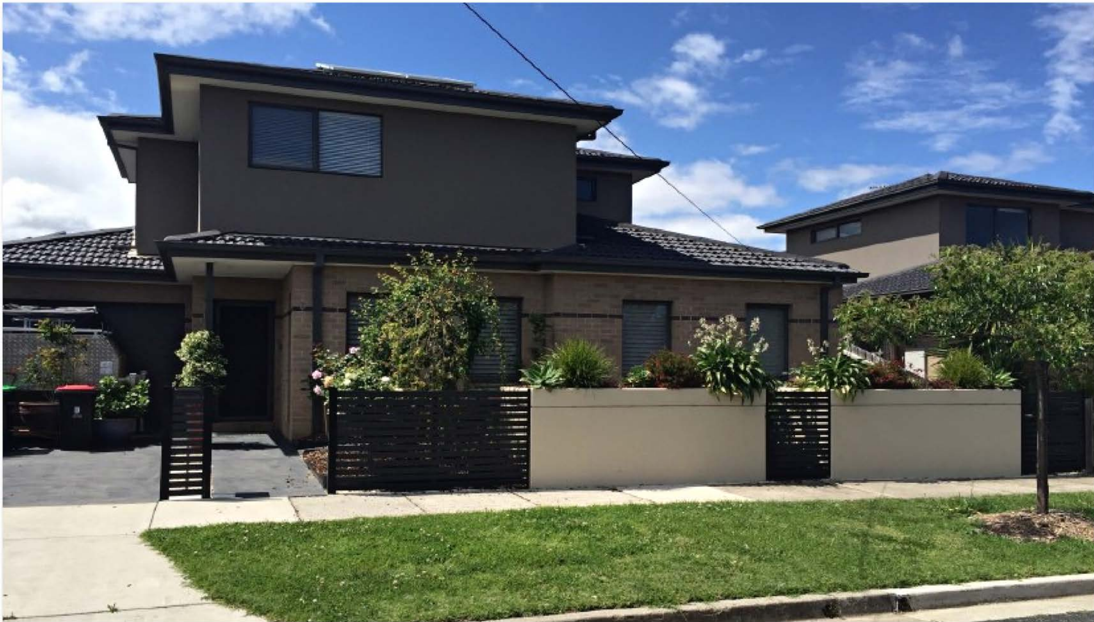
A simple front fence and water retention installation which also provides a noise barrier and unrestricted height privacy through plant selection. Plants 0.4 – 1.0m tall become 1.4 – 2.0m of privacy.
